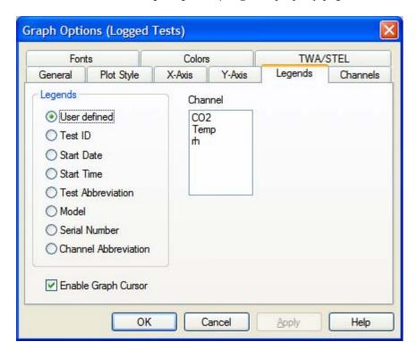
When enabled, the cursor coordinates of any point on the graph may be measured by moving the mouse pointer to the desired location and reading the results in the Status Bar window at the bottom of the Graph Screen.
