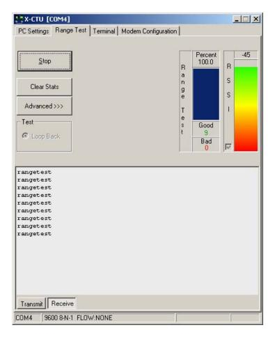
The test command will be looped between the PC Radio Modem and Instrument Radio Modem, and the signal strength is measured and displayed. With this information, the user can adjust the Instrument location and antenna direction, to provide the most reliable communication link. Having a clear line of sight between Radio Modems is critical for achieving the best possible signal.
