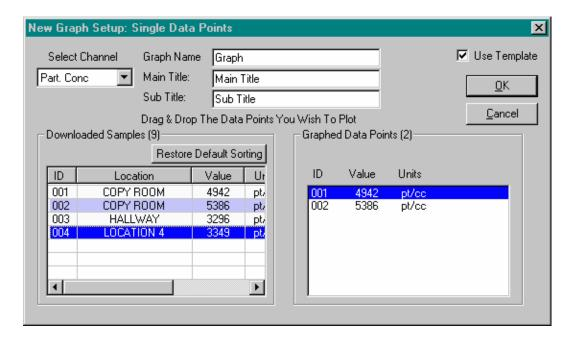
Both forms of dialog box allow the graph to be based on a previously saved template.
